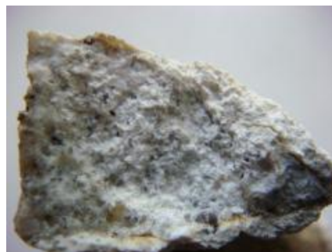
Cross section of existing pointing mortar
