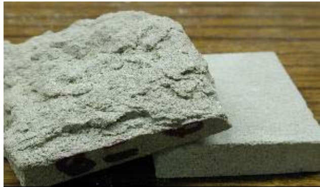
Reigate T.1, laboratory induced scaling (freeze/thaw testing)
