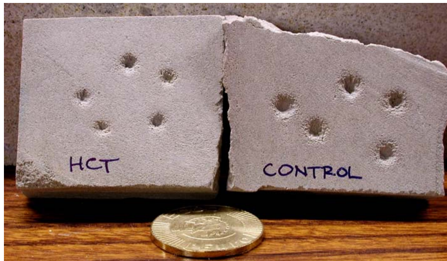
Figure 2: Microabrasion, 5 craters each specimen
