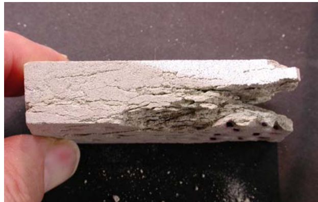
Reigate T.1, laboratory induced incipient scaling (freeze/thaw testing)
