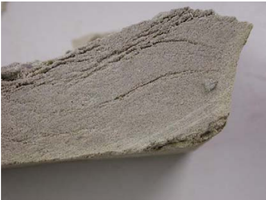
Reigate A.1, cross section showing incipient scaling
