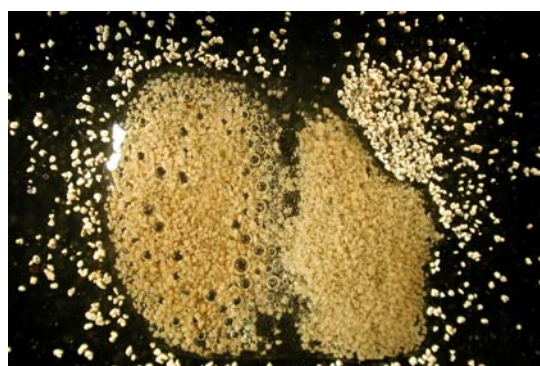
Reaction with .09M sulfuric acid, pH 1.1
