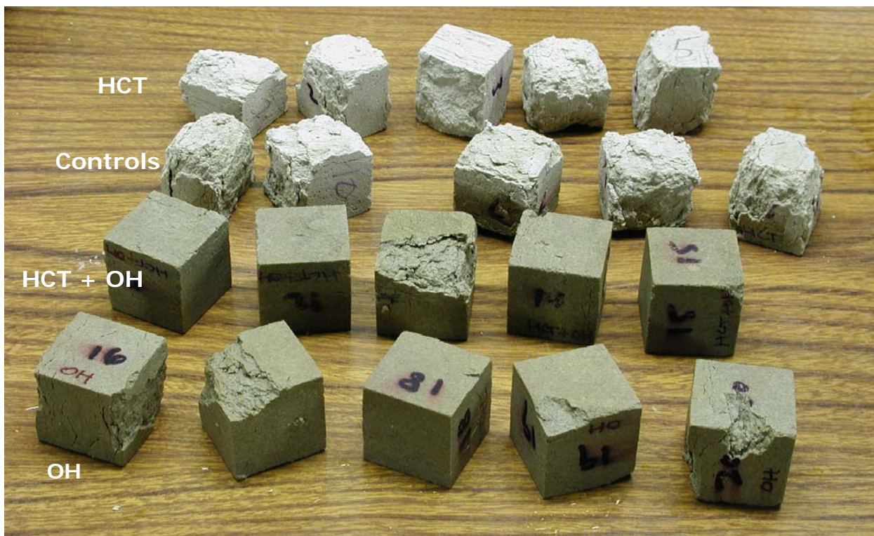
Figure 4: Back to front: HCT (dry) at cycle 34, controls (dry) at 26, HCT + OH (wet) at 50, OH (wet) at 50
