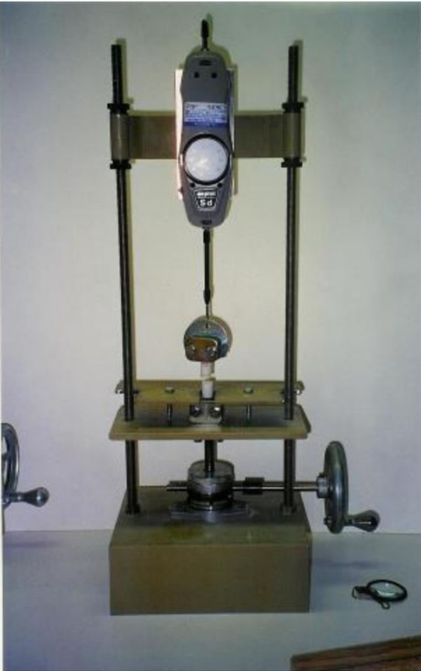
Testing surface-coupled cores in tensile failure
