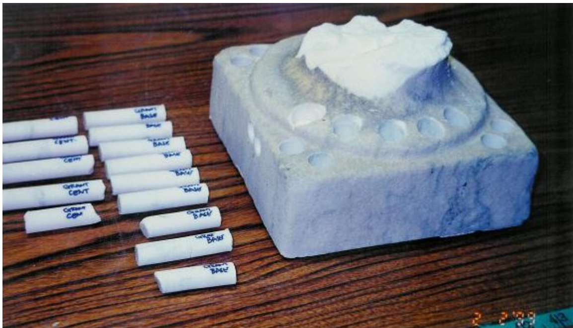
Cores taken from the base of the baluster
