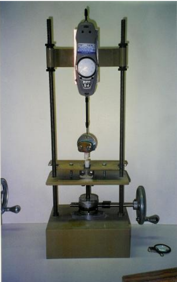
Testing surface-coupled cores in tensile failure
