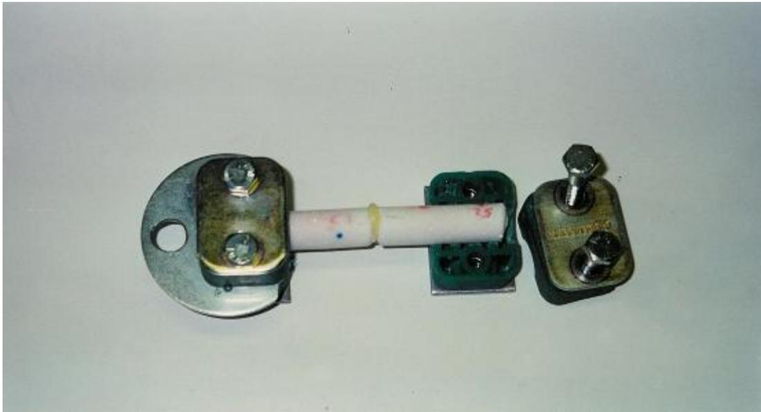
**Surface-coupled cores secured with pipe clamps**
