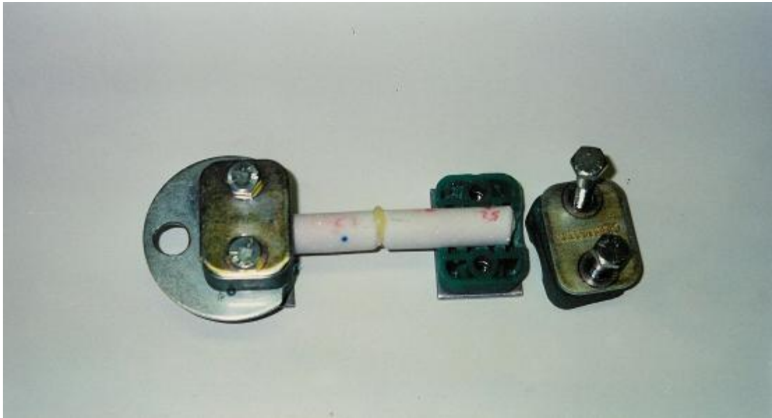
Surface-coupled cores secured with pipe clamps
