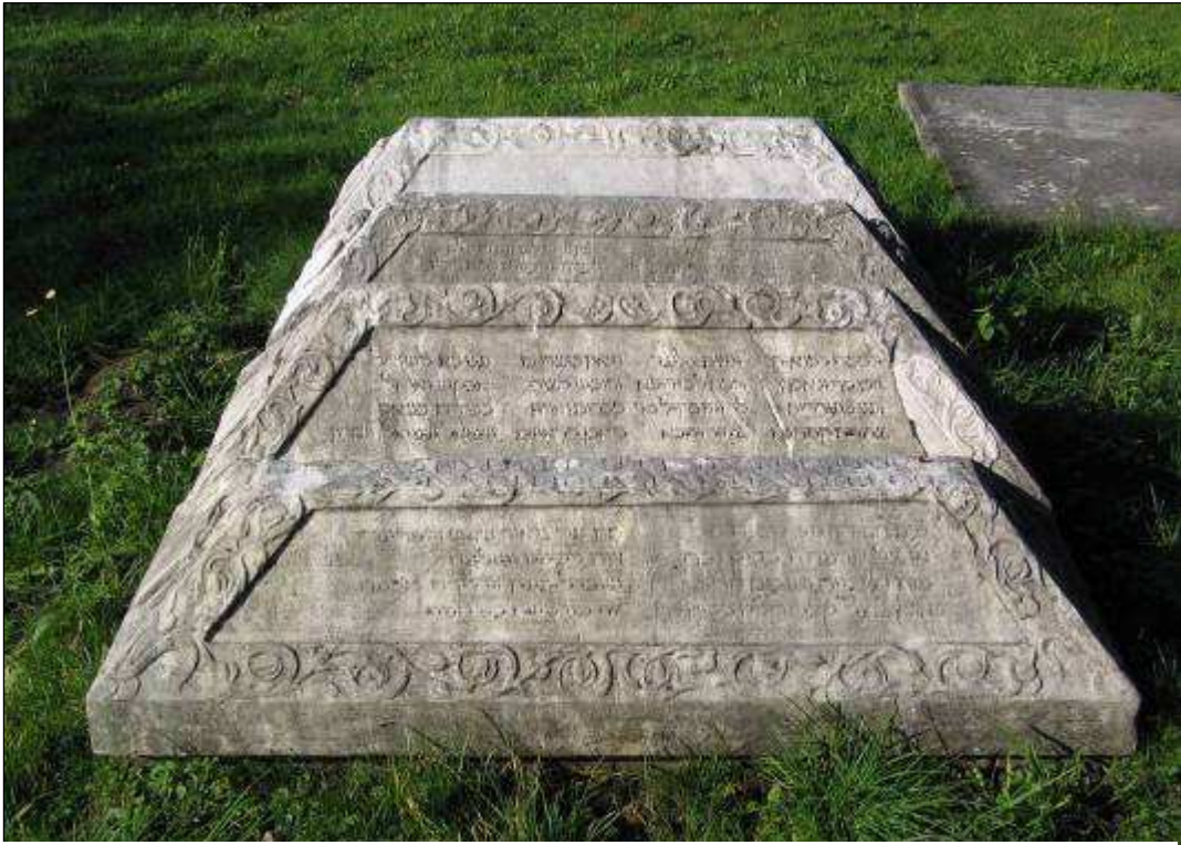
The second testgroup at October 19th 2004, not long after they were pressure-washed.
